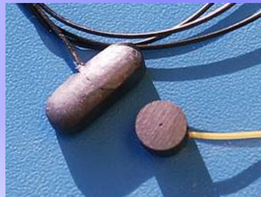
Drug-shaped Electrodes for Predicting Initial Dissolution Rates
